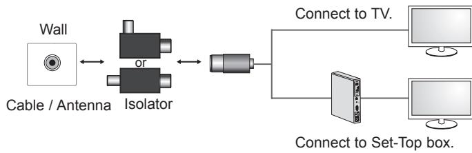
Connect one end of the isolator to cable/antenna jack and the other to TV set or set-top box.
